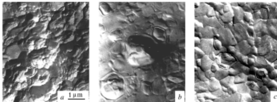
Fig. 5. Morphology of the silicon-doped film upon deposition (a) and prolonged (b) and fast (c) treatment.
